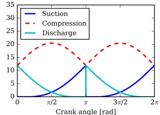
**Calculate volume and volume derivative of working chambers**
